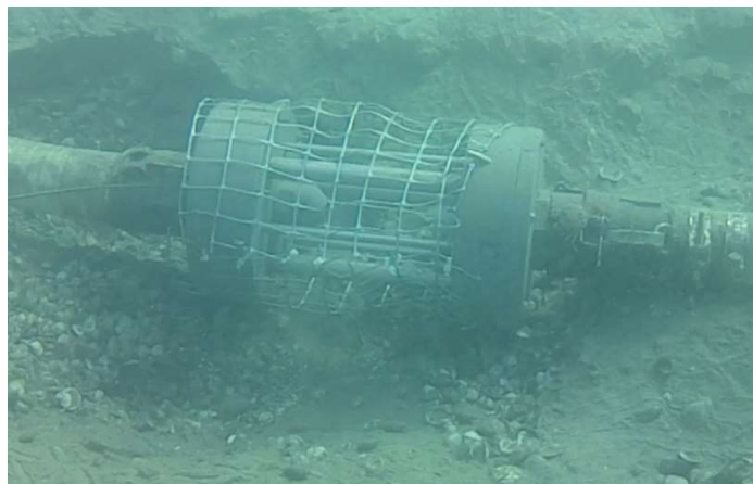
Figure 3. a) Sketch of the ejector, and b) underwater picture of the ejector in operation.
