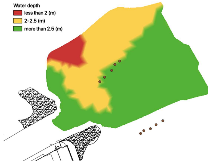
Figure 8. Colormap of water depth for specific ranges (more than 3.0 m, between 2.0-2.5 m and lower than 2.0 m) on 11 th of September 2020. The red circles indicates the GPS reference of the mooring points of inlet and outlet ejectors pipelines. The ejectors are installed between the inlet/outlet mooring points, as showed in Figure 2.
